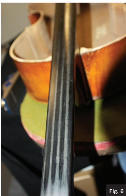
The deep grooves in a fingerboard are caused by strings; hollows are from finger wear.
